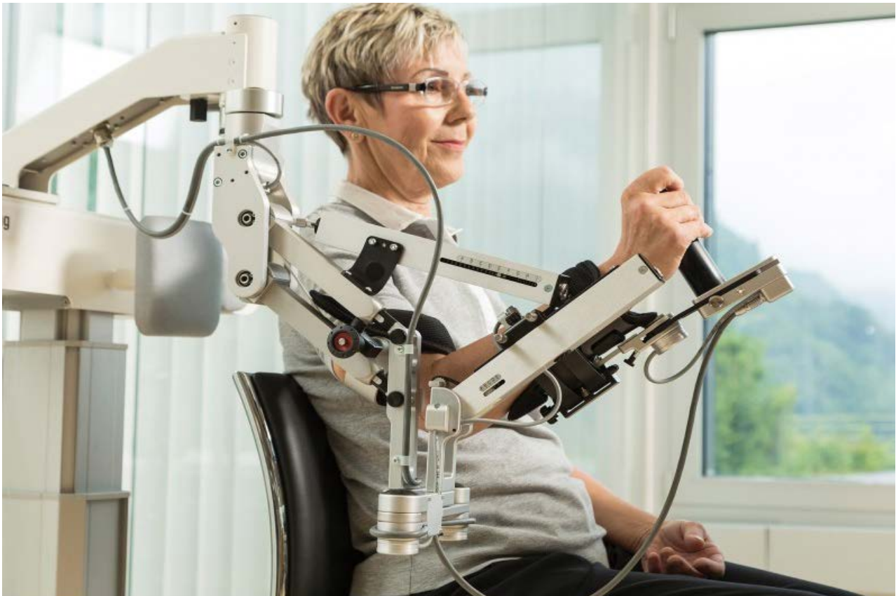
Illustration 22. Device with an advanced spring mechanism for rehabilitation of the upper limb 20 .
