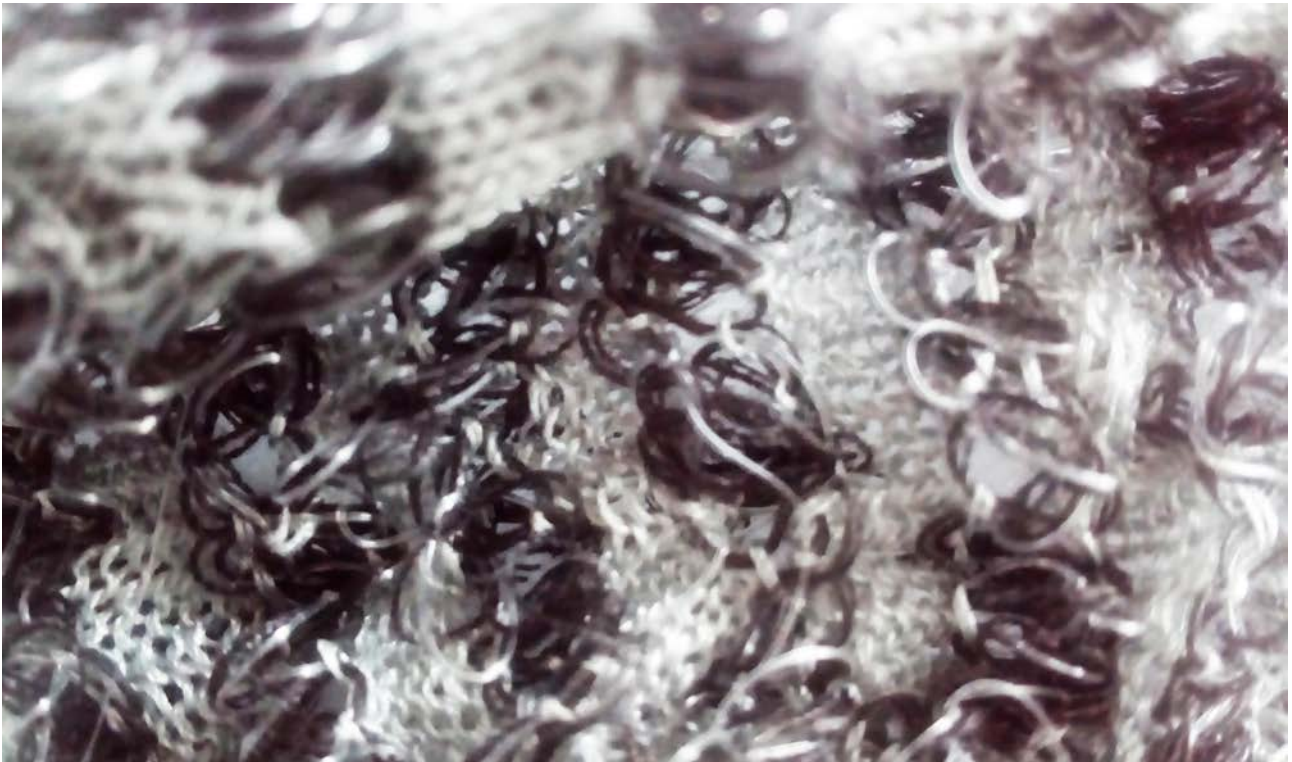
Illustration 37. Trial surface knitted with the use of polyamide yarn.
