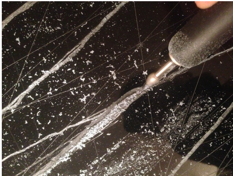
Illustration 5. Work on the matrix using the multifunction dremel tool.
